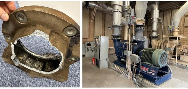
Figure 3 – Catastrophic Failure of Centrifugal Blower
