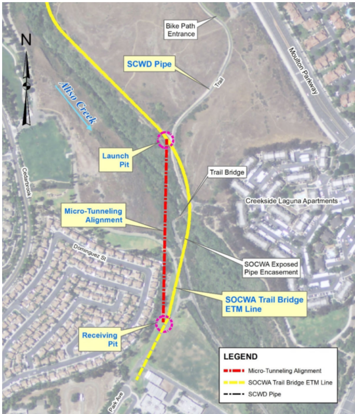
Figure 2 – Approximate Alignment of Microtunneling the Vulnerable ETM Segment
