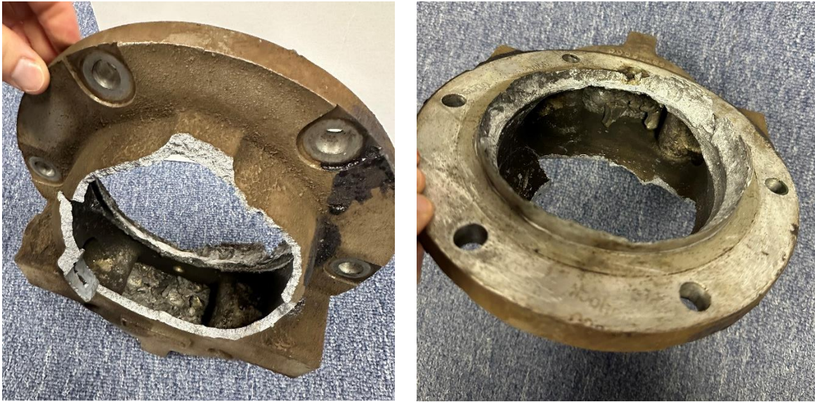
Figure 5 – Catastrophic Failure of Centrifugal Blower
