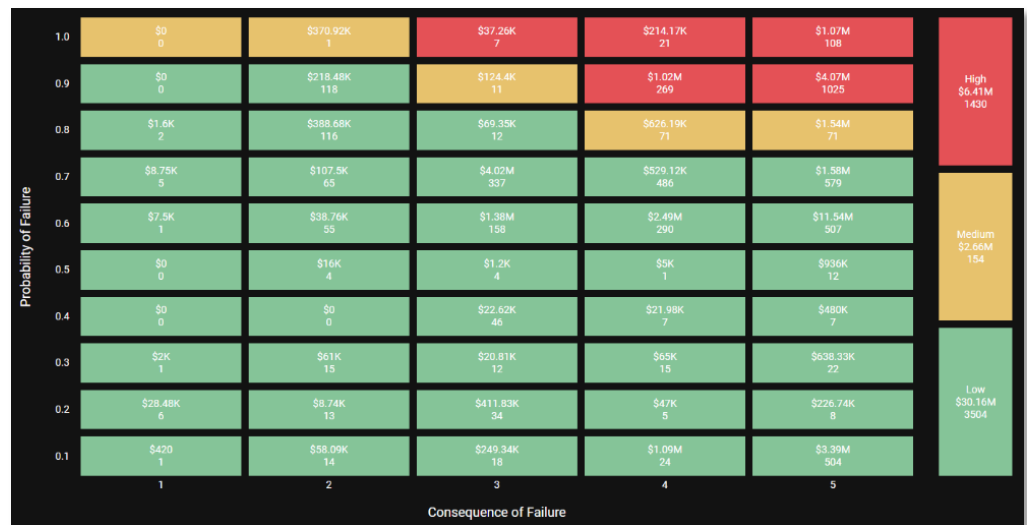
Example of a risk matrix window showing the distribution of assets into different risk levels. Each cell in this matrix shows the number of assets with the same risk level and their associated total replacement cost.
