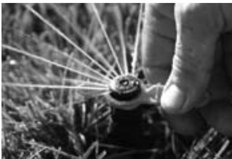
Rotating nozzle sprinkler head.
