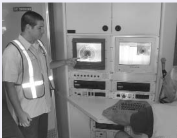
Ty Banagas, in the computerized video inspection van control room viewing the inside of a pipe.
