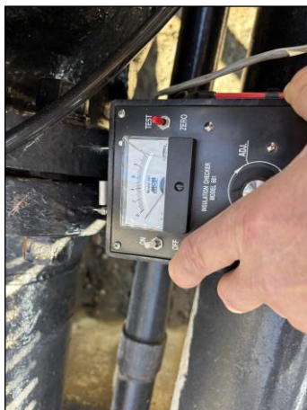
Figure 6 - Model 601 Insulation Checker
