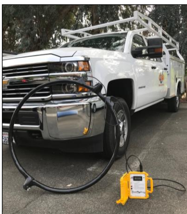
Figure 4 - Swain Inductive Ammeter Current Measurement System
