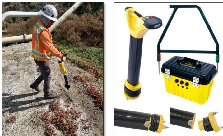
Figure 5 - Vivax Metrotech vLocDM2 Current Mapper
