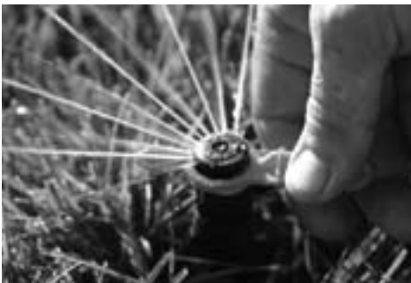
Rotating nozzle sprinkler head.
